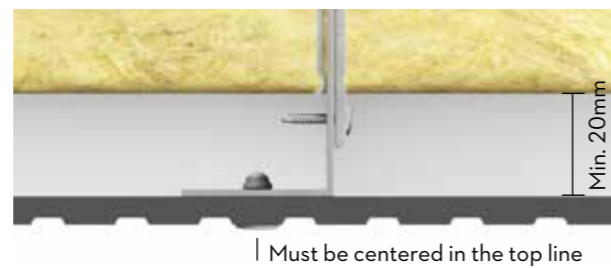
Fig. 2. Cembrit Patina Inline installation on L profile.
