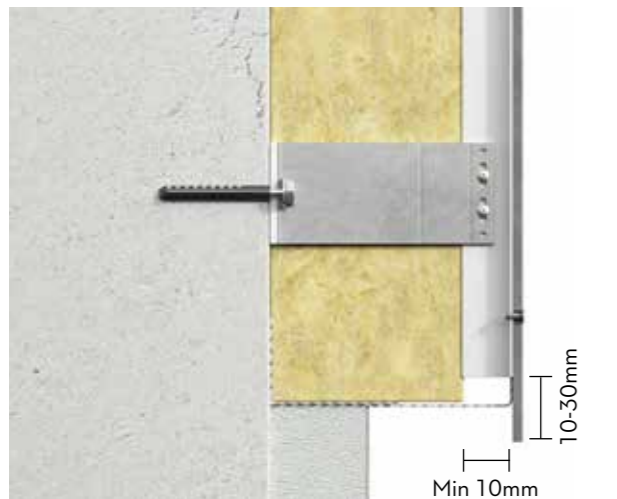
Vertical view: Plinth construction
